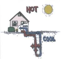
Complete First floor and second floor ducted "5 ton" Closed Loop Vertical Bore Geothermal Heating and Cooling system, including;
