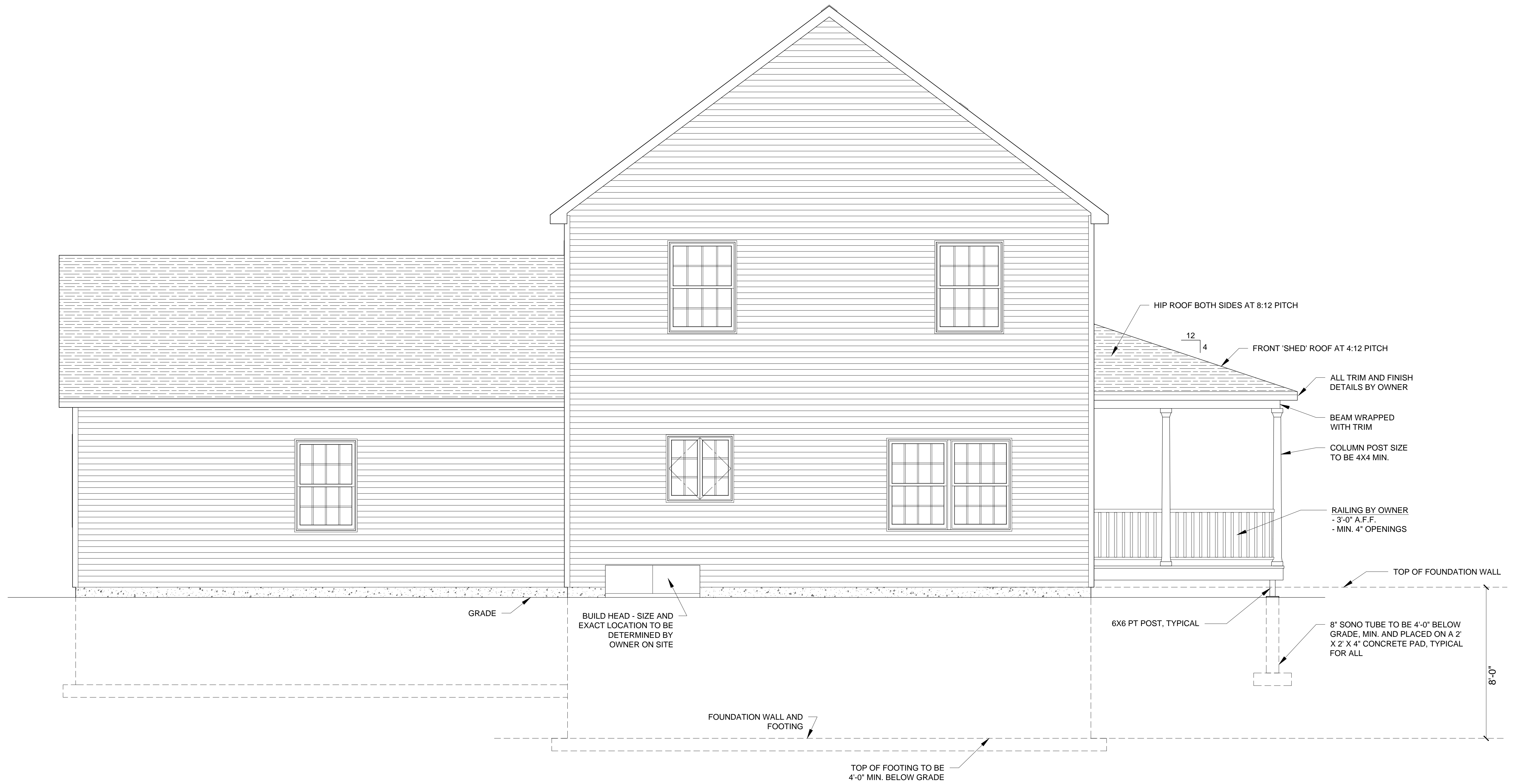
1 BACK ELEVATION 3/8" = 1'-0" (WHEN PRINTED AT 24"X36")
