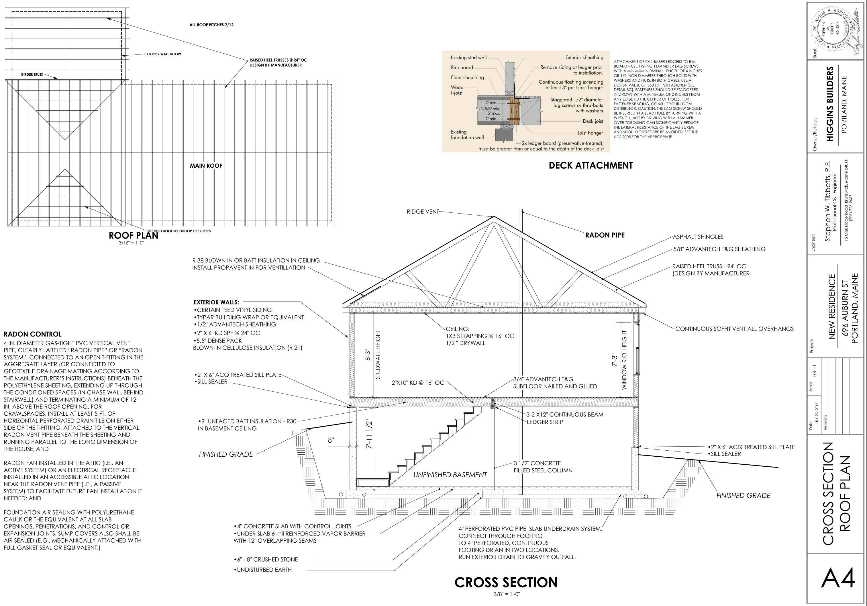
FOUNDATION AIR SEALING WITH POLYURETHANE CAULK OR THE EQUIVALENT AT ALL SLAB OPENINGS, PENETRATIONS, AND CONTROL OR EXPANSION JOINTS. SUMP COVERS ALSO SHALL BE FULL GASKET SEAL OR EQUIVALENT.)
