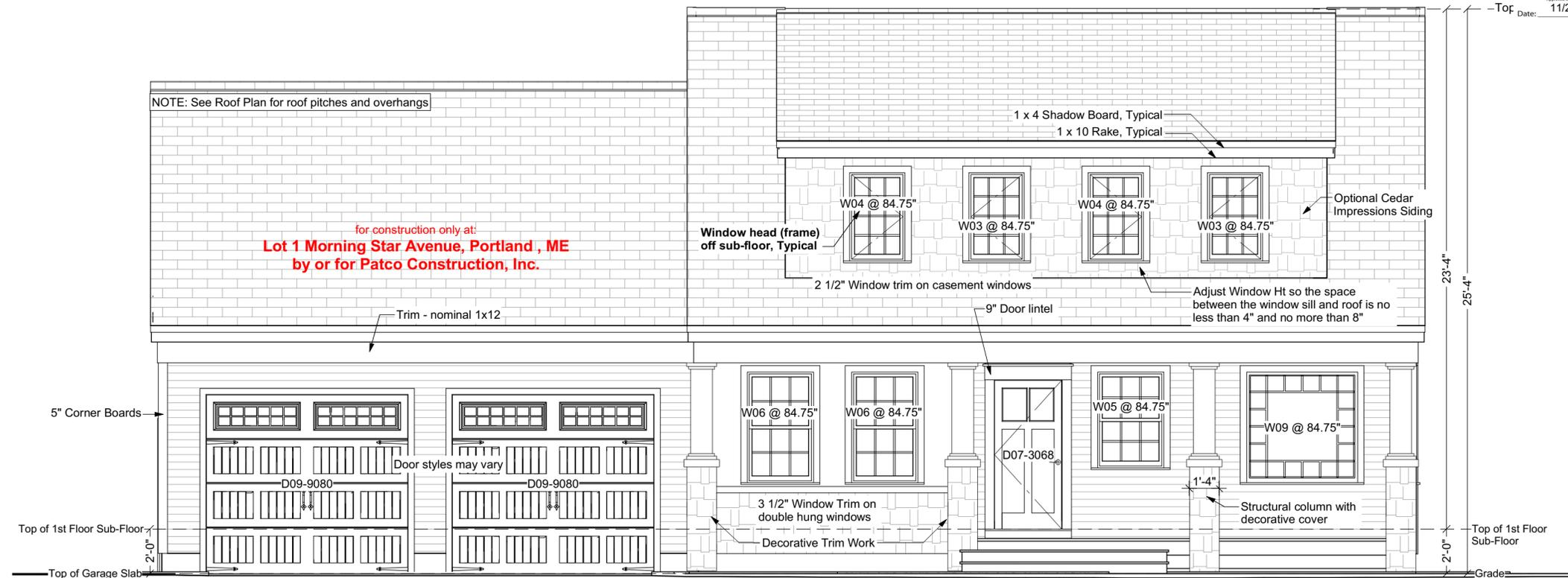
Garage slab height may vary. If garage slab height is lower than shown, consult Artform for aesthetic direction. Taller garage doors, transoms, lintels and/or additional frieze boards may be required to achieve desired look.
