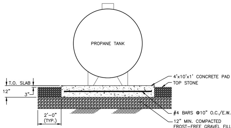
**CONCRETE PAD SECTION DETAIL**
