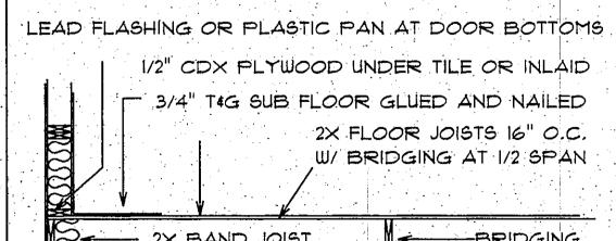
EXT WALLS PERPENDICULAR TO JOISTS
