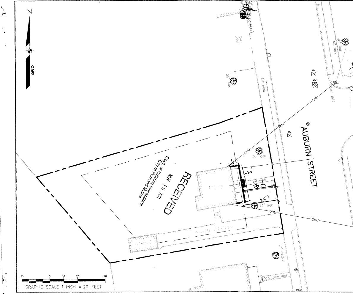
Front 23.5' Allowed under Front 23.5' Allowed under (A-425 - of (A-425 - of (A-425 - of (A-25'+ Show PAR. 25'-25'+ Show Side; 8'm - wellow 8' ø نĐ B84-A-16 **OVERALL SITE PLAN PROPOSED PORCH** ⊡Mf FOR MATTHEW EK & CANDACE ANDERSON-EK 424 AUBURN STREET, PORTLAND, ME 04103
