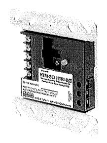
The interface module reports the status of the (NO) or (NC) contact to the control panel. Model HTRI-S can only monitor and report the status of the contact, while Model HTRI-R incorporates an addressable Form C relay.
