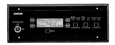
The Model FS-RD2 Remote Display is used for annunciating system events remotely from the fire alarm control panel on the FireSeeker FS-250 system. The FS-RD2 will mimic the system status LEDs and the 80-character event message found on the main system panel. The 4 x 20 LCD backlit display will illuminate upon receiving any event from the system, or upon pressing any button on the FS-RD2.
