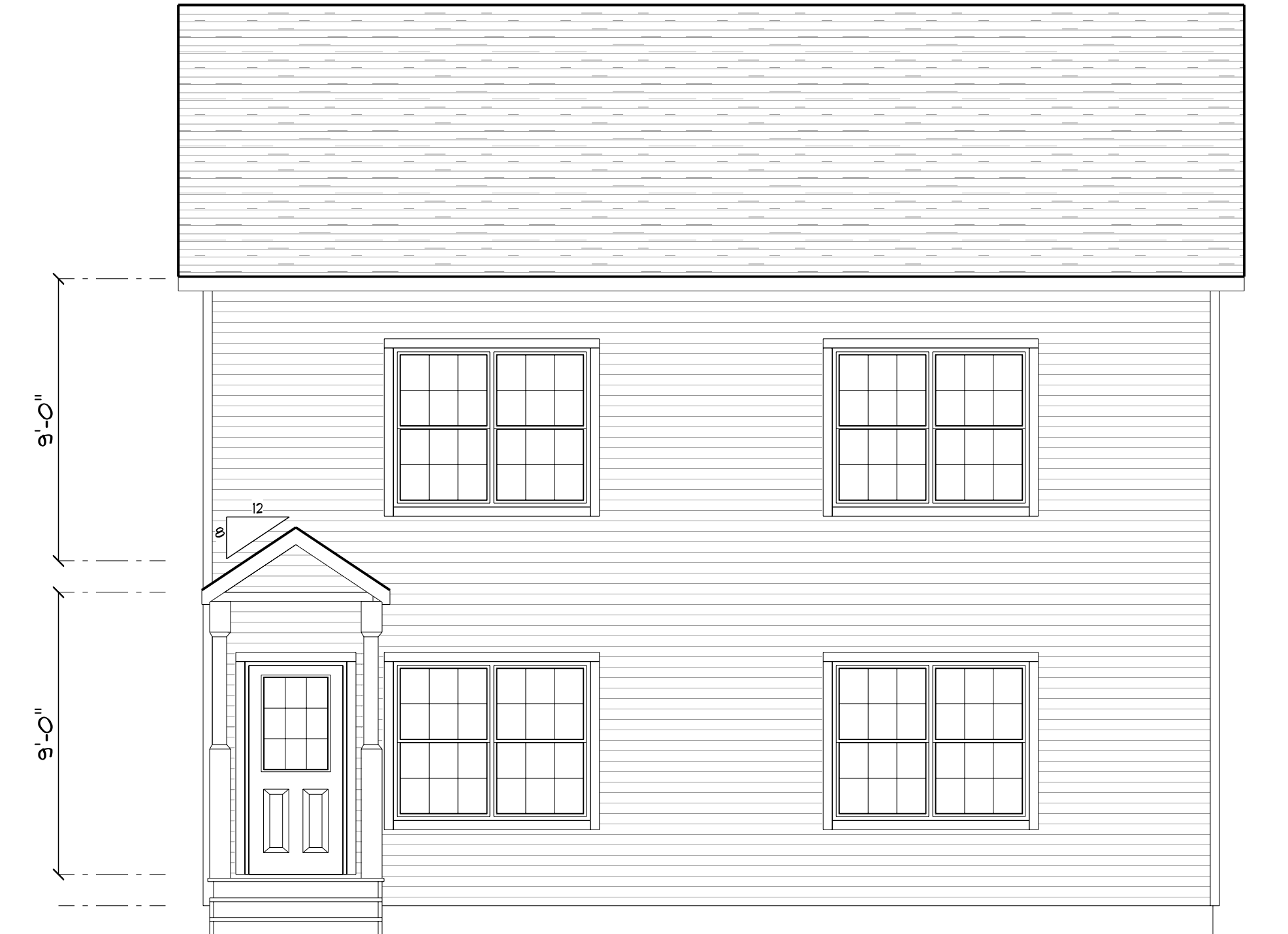
FRONT ELEVATION SCALE: 1/4" = 1'-0"
