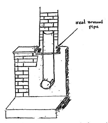
Place stove on hearth, slide stove back toward short piece of pipe. Ease pipe out to connect onto stove outlet. Secure with screws. Slide stove back against fireplace.
