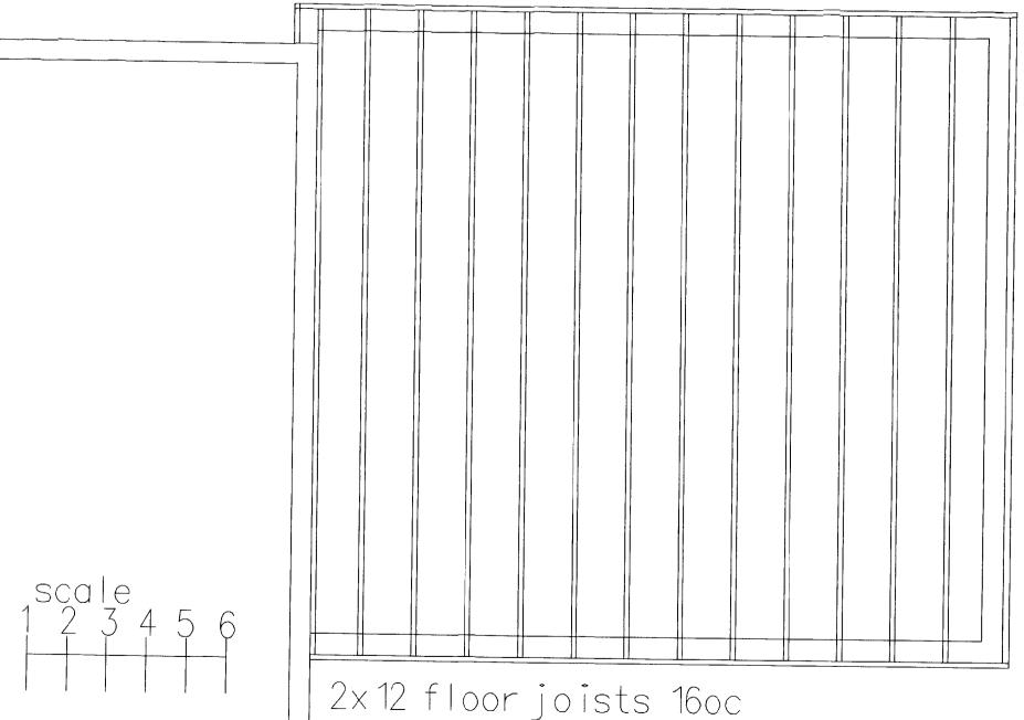
2x12 floor joists 16oc with 2rows of solid blocking
