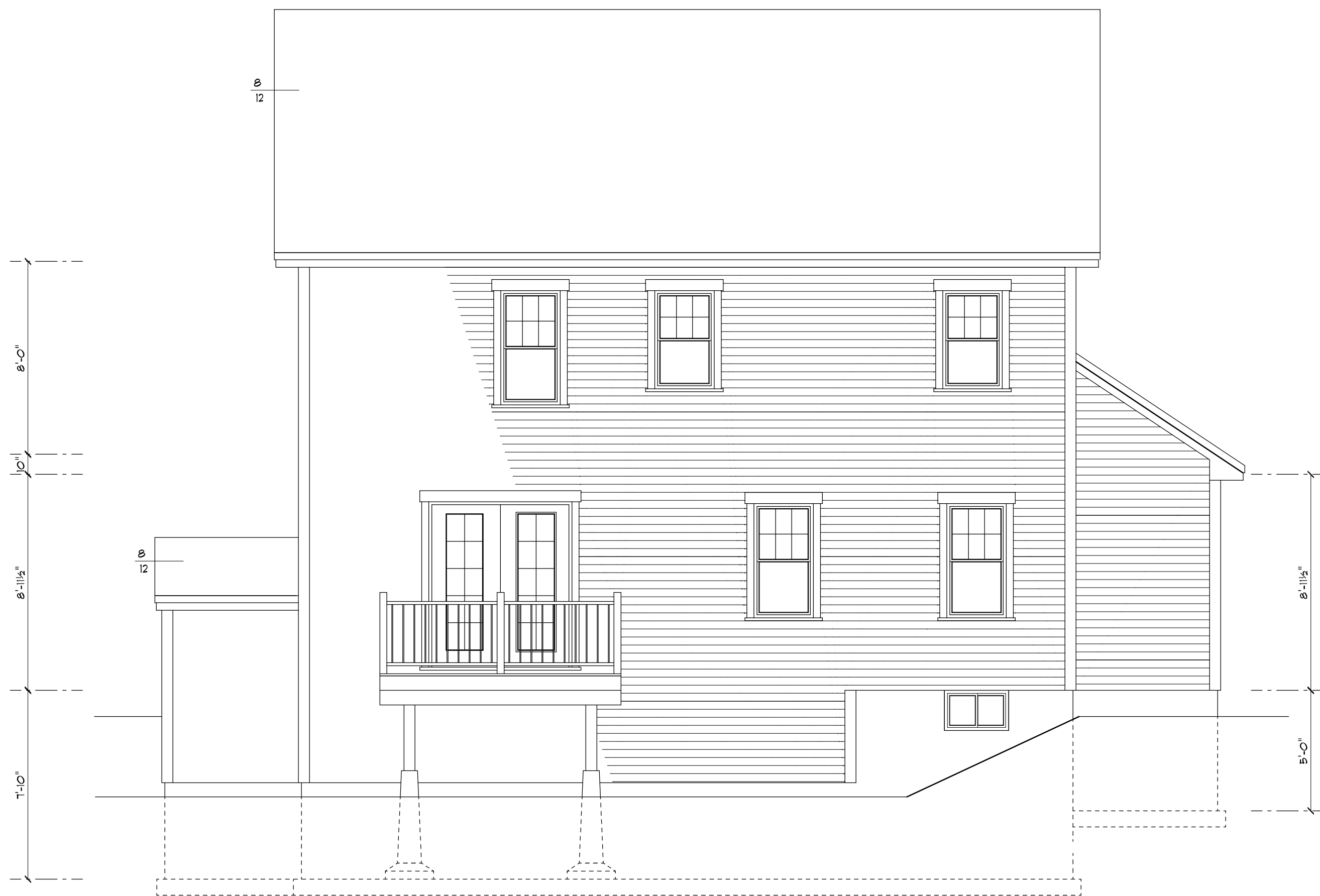
REAR ELEVATION SCALE: 1/4" = 1'-0"
