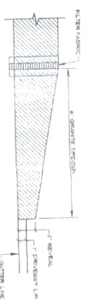
TYPICAL TIPDOWN CURB INSTALLATION NOT TO SCALE
