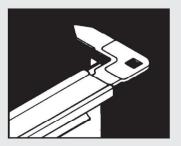
In the field insert a corner piece into the angle at the male end of the Pittsburgh Lock
