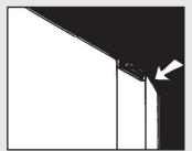
Notch the "hammer edge" of the female Pittsburgh Lock 1/4" on a 45 degree angle as shown
