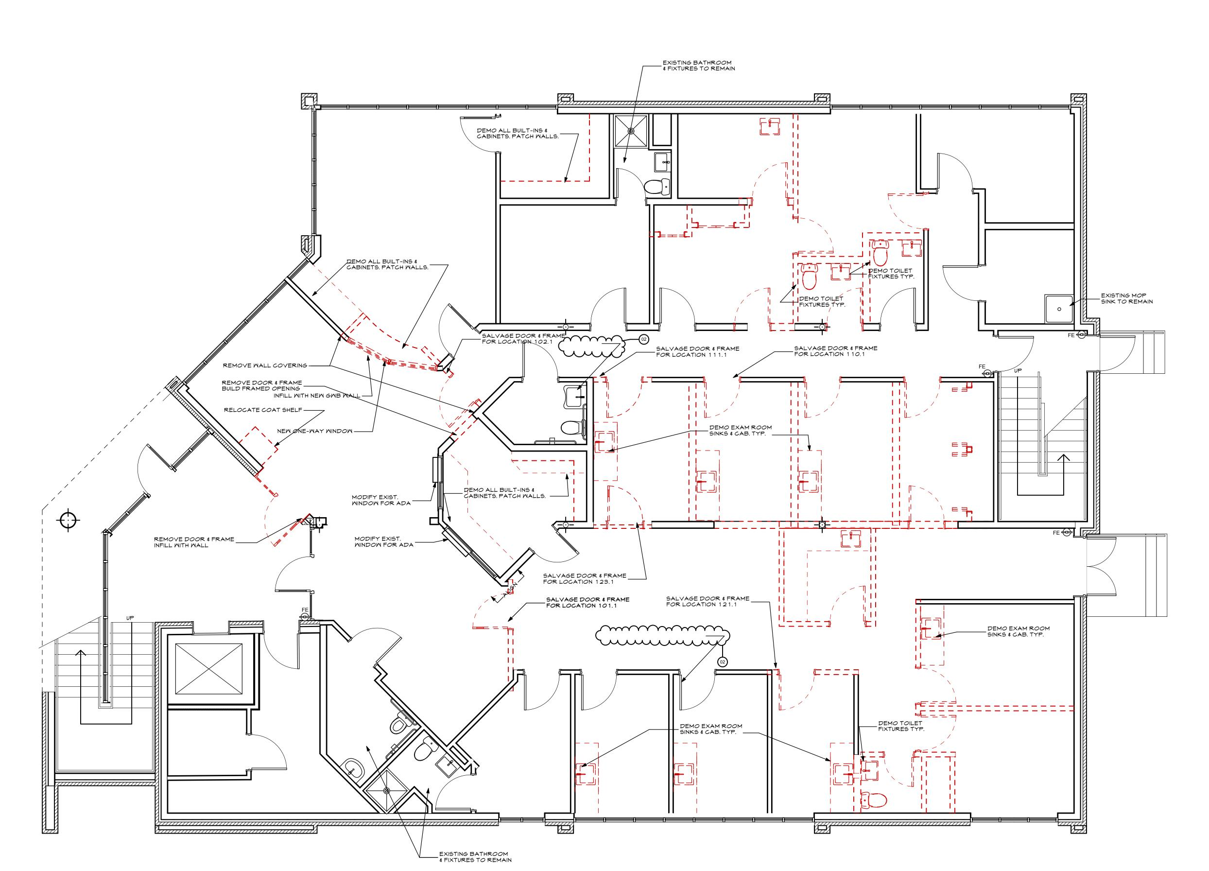
LEGEND: WALL TYPE 1 TYPICAL SEE SHEET NO. A4.1 **NEW WALL** DIMENSION TO THE FACE OF STUD UNLESS OTHERWISE NOTED EXISTING WALL TO REMAIN EXISTING CONSTRUCTION TO BE
