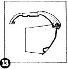
firmly in place. Bring the lower connector down into place under the top rails by spreading the sides out completely, as shown in diagram 11, and **gently** stretching it across and down, as shown in diagrams 12 and 13.
