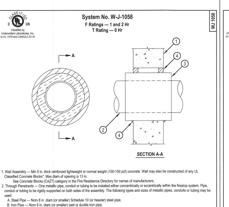
3. Pipe Covering — Nom 2 in. thick hollow cylindrical heavy density (min 3.5 pcf) fiberglass pipe covering with an all-service jacket. Pipe covering
