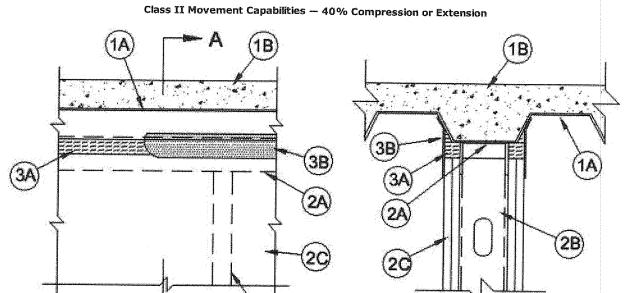
1. Floor Assembly — The fire-rated fluted steel deck/concrete floor assembly shall be constructed of the materials and in the manner described in the individual D900 Series Floor-Ceiling Design in the UL Fire Resistance Directory and shall include
