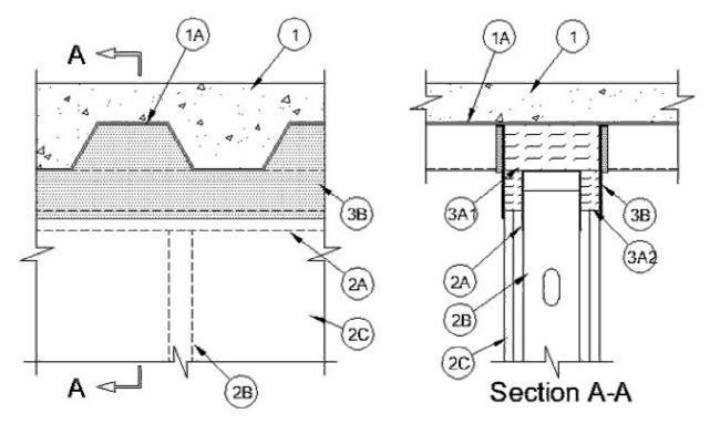
1. Floor Assembly — The fire rated fluted steel deck/concrete floor assembly shall be constructed of the materials and in
