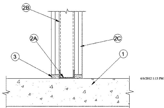
1. Floor Assembly — Min 4-1/2 in. thick reinforced lightweight or normal weight (100-150 pcf) structural concrete. Floor
