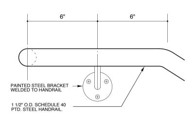
TERMINATION ELEVATION AT TOP OF STAIRS
