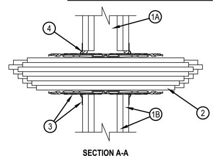
. Wall Assembly —The 1, 2, 3 or 4 hr fire rated gypsum board/stud wall assembly shall be constructed of the materials and in the manner described within the individual U300, U400, V400 or W400 Series Wall and Partition Designs in the UL Fire Resistance Directory and shall incorporate the following construction features:
