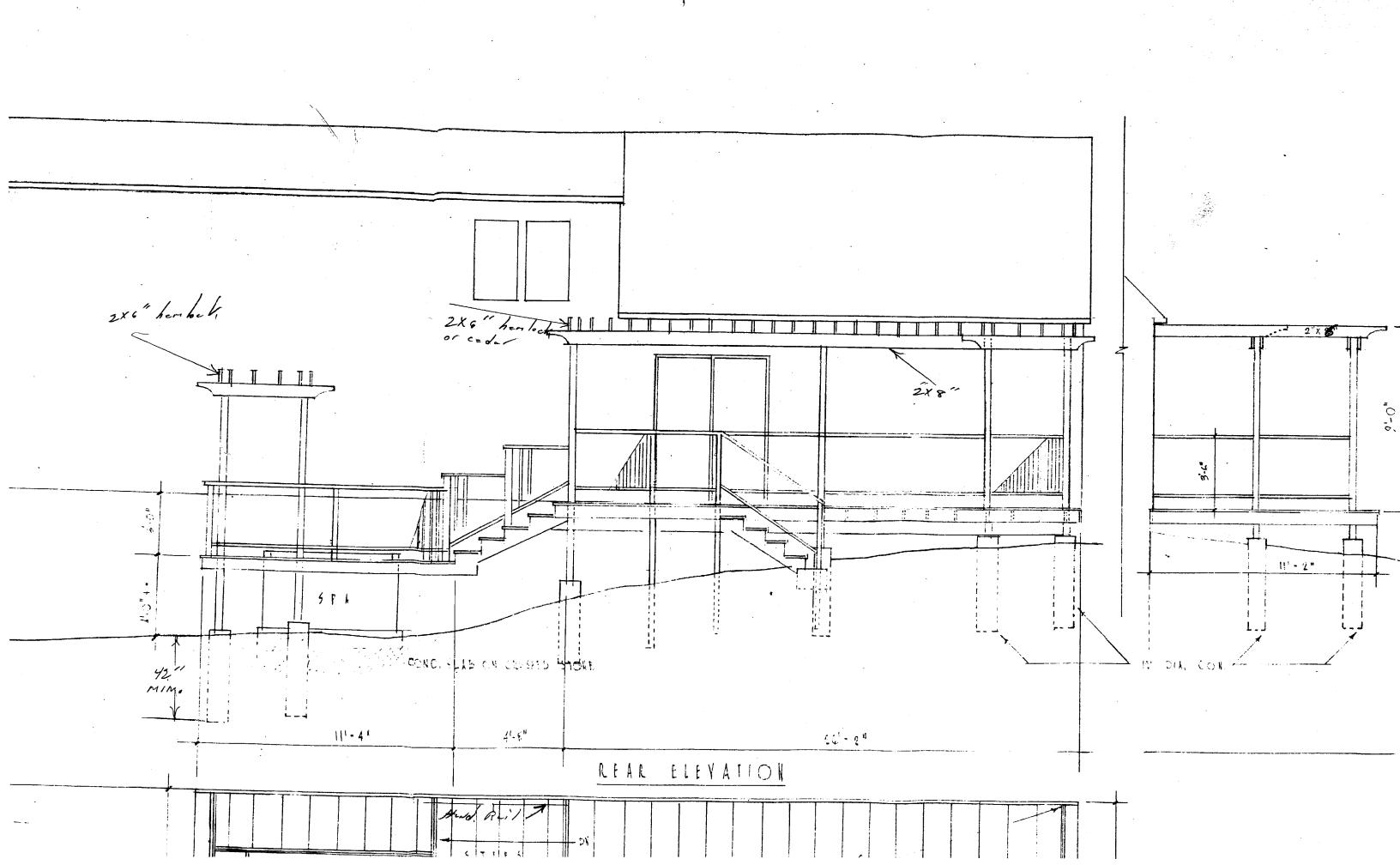
Notes; 11) Deck joists are to be 2x8 p.t. 16 O.C. 12) All rails, hardrails and steps to conform to BOCA Not. Blyg Code 129 section 1014.6 + 1022.2.3
