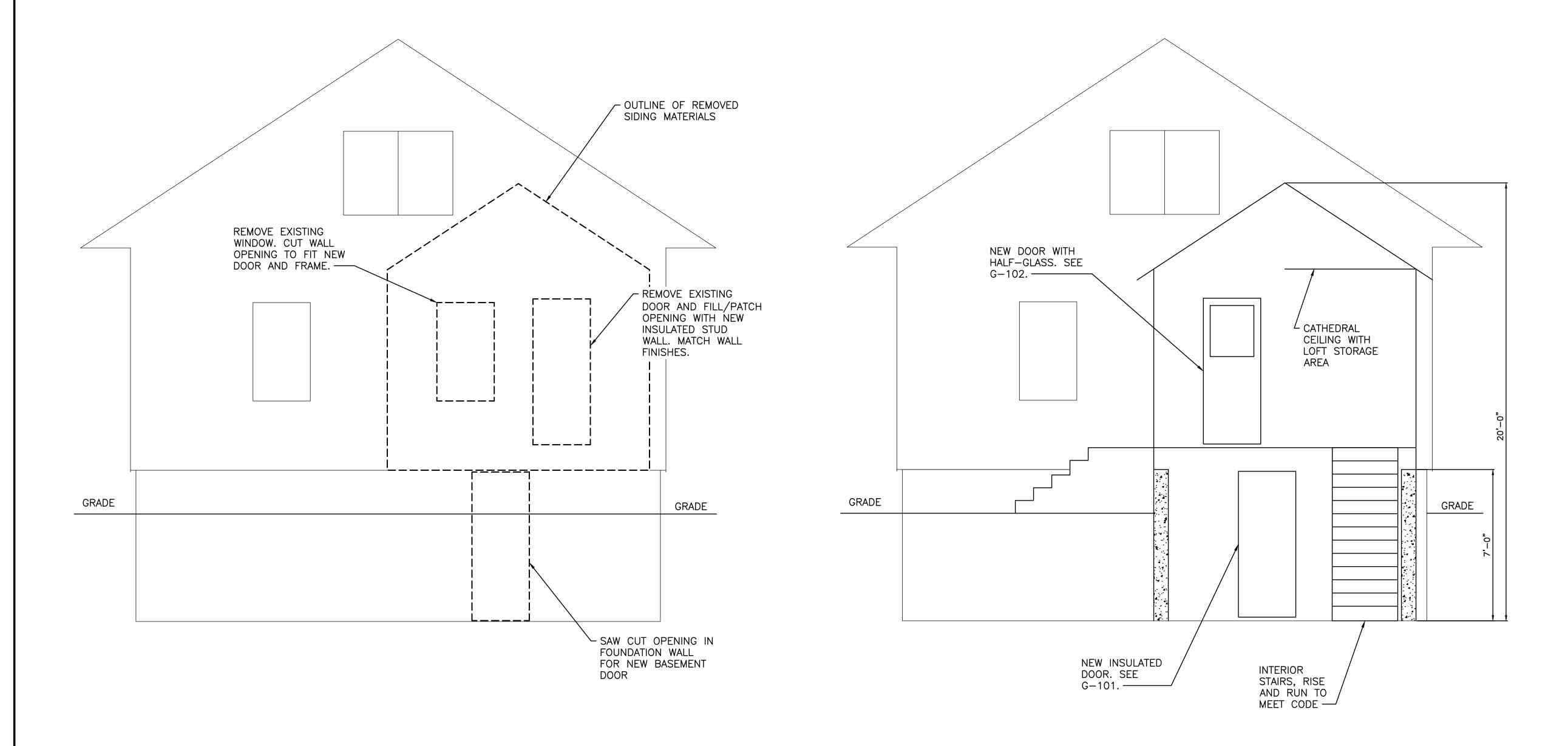
ADDITION SECTION — DEMOLITION SCALE: 3/8" = 1'-0"
