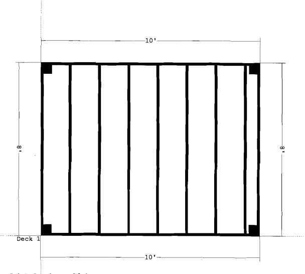
Joist Spacing = 16 in. o.c. Baluster Spacing = 3 3/4" Toe Spacing = 3 3/4" Railing Height = 36" The Home Depot # 2401
