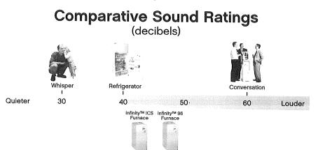
Carrier manufactures gas furnaces that are among the quietest in the industry. We test our products in a sound laboratory specifically built to semble a typical residence. Sound level recordings produced at steady state, low fire operation (the most common operating condition), measured 3 feet from furnace. Other sound levels, mentioned for comparison, as published at http://www.nidcd.nih.gov/health/hearing.ruler.asp.
