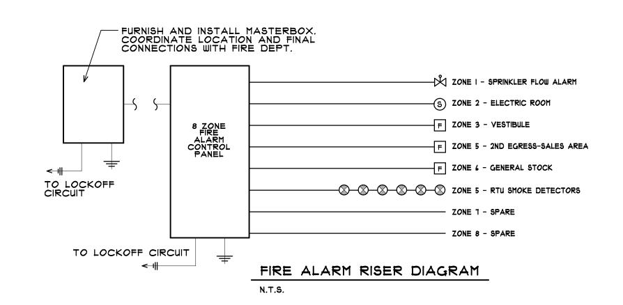
LEGEND DUCT SMOKE DETECTOR AT EACH HVAC UNIT RETURN DUCT (SHUT-DOWN UNIT WHEN SMOKE IS DETECTED) (S) SMOKE DETECTOR (CEILING MOUNTED) SPRINKLER SYSTEM FLOW ALARM F FIRE ALARM PULL STATION 9 42" A.F.F.
