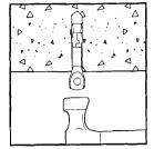
Set the anchor with a prying action using a claw hammer.
