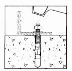
Tighten the anchor by turning the nut 3 to 4 turns or by applying the guide installation torque from the finger tight position.
