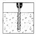
Blow the hole clean of dust and other material. Position the washer on the anchor and thread on the nut.
