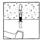
Tighten the anchor by turning the coupling 3 to 4 turns or by applying the guide installation torque from the finger tight position.
