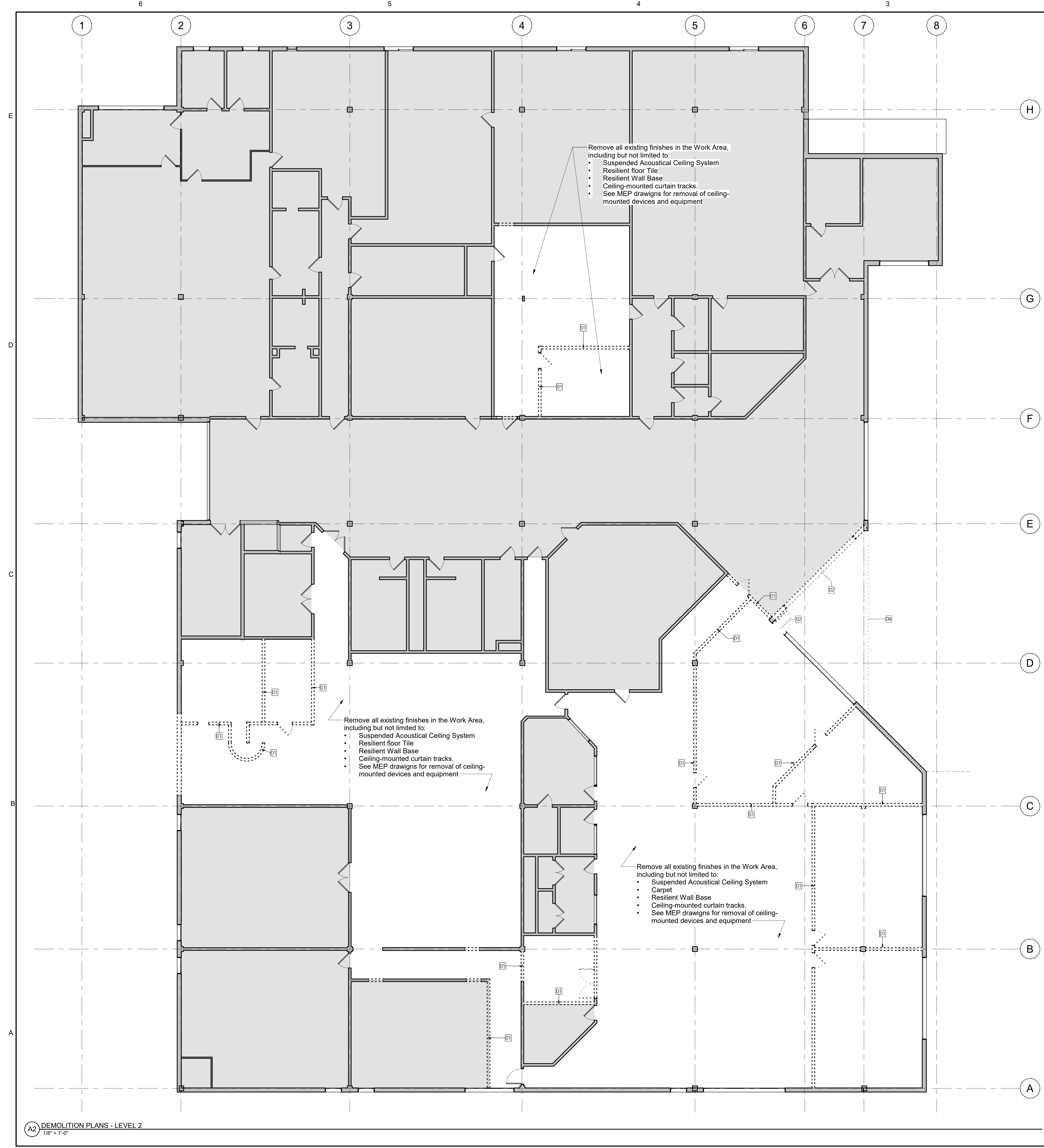
A1 DEMOLITION PLAN - LEVEL 1 1/4" = 1'-0"
