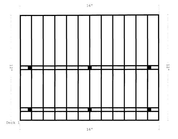
Joist Spacing = 16 in. o.c. Baluster Spacing = 3 3/4" Toe Spacing = 3 3/4" Railing Height = 36" The Home Depot # 2401 245 RIVERSIDE STREET, PORTLAND, ME 04103 (207) 761-0600 Sat Apr 05 13:47:00 2008 MARGO CLOUGH RTS DECK 262384
