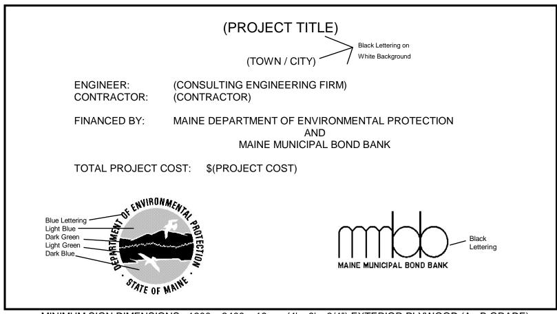
MINIMUM SIGN DIMENSIONS: 1200 x 2400 x 19mm (4' x 8' x 3/4") EXTERIOR PLYWOOD (A - B GRADE) MINIMUM LETTERING DIMENSIONS: 2"
