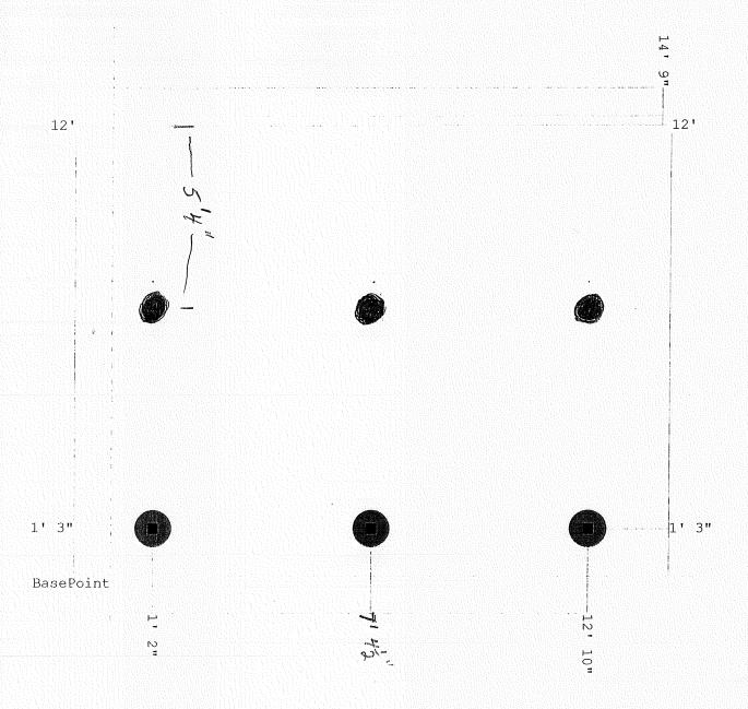
Proposed Deck Gina St. Claire 27 June 08 81 Ruby Lane Revo Page 5of7 15 =1' 2x4 Between Post + under rail to a Hack rail spindles 2x4 Between Wast + under Kescrew Syx6 Dectrin 1 attached to from by 3'Deck Syx6 Dectrin 1 -4x4support post 2×4 Roil attached to top of post w 3 Deck Screw 2×2×41" Railing Spindles Attached w 2'z Deck 2×2×41" Railing Spindles Attached Screw 36 ec! irface 8" carriage Bolts 4x4x42" V334 Sporing Max o Top 1/2 =1 fRailing
