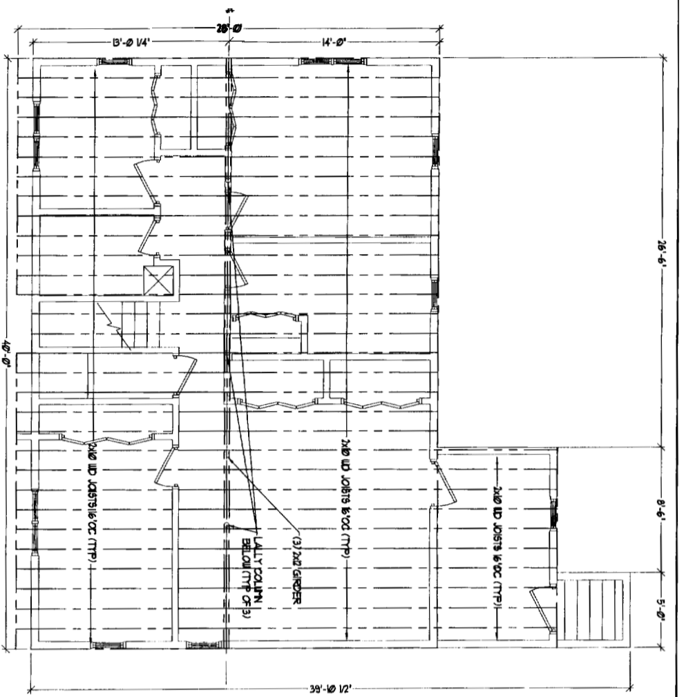
1 FIRST FLOOR FRAMING PLAN SCALE: 1/4" = 1'-0"
