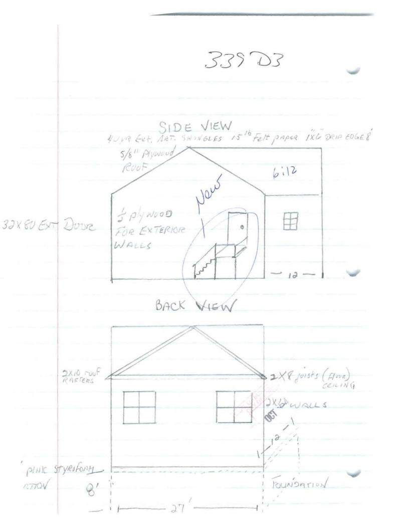
339 D3 - 44 -41" 38" 82" 82 872 36×80 EXT. Metal door Header 2×6 W/ 5 plywood nailed + glued
