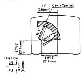
Before drilling the flue hole, check for water and gas pipes as well as electric cables. Use a 3 1/8" (80mm) drill for hole through wall.
