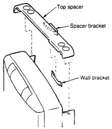
Replace top spacer, clipping the spacer into the wall brackets at the same time as attaching it to the heater. Secure top spacer with the screws provided. THE HEATER IS NOW SECURED TO THE WALL.
