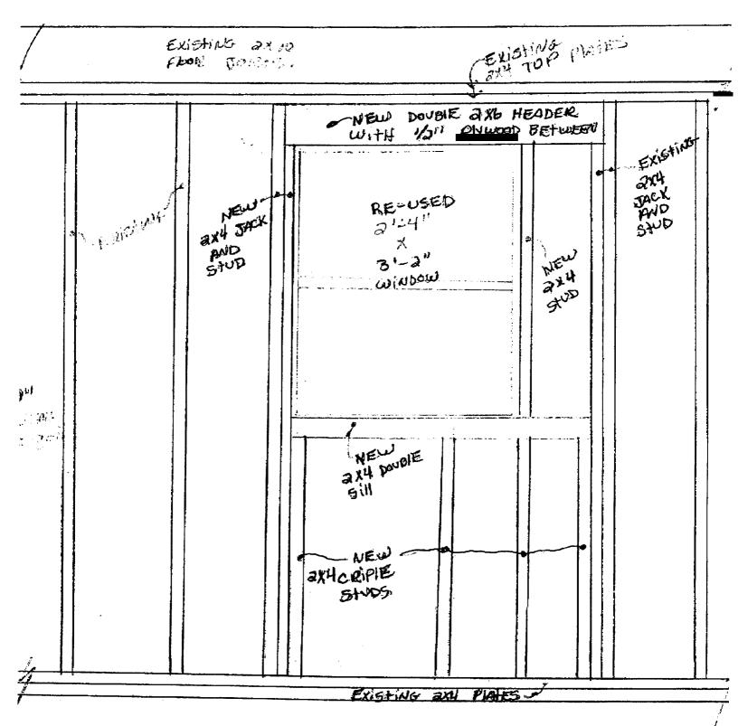
VIEW FROM INSIDE, EXISTING WINDOW 15 BEIOS MOUED 12" TO THE LEFT BY ENLARGING EXISTING ROUGH OF ENVIOL. NEW OPENING BHOOM with wincom IN FINAL Position.
