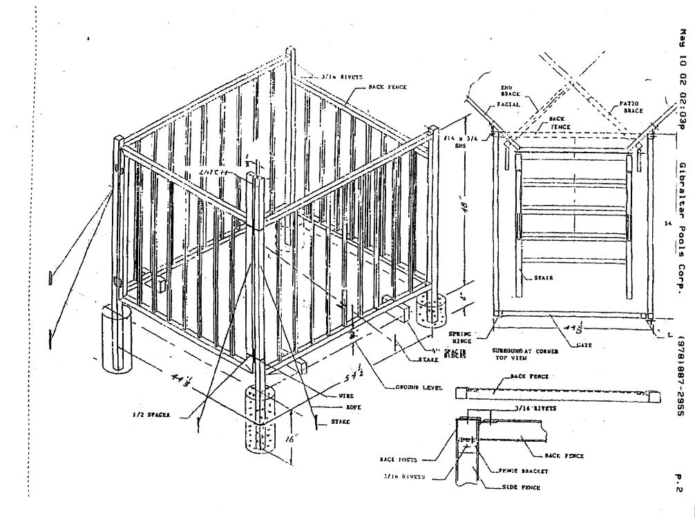
Lock To be 57" High 51 des to be 48" hight Gate 4'opening Post \*Will have self closer \* Gate will swing away from pool & latch will be above 54"
