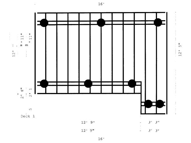
Joist Spacing = 16 in. o.c. Baluster Spacing = 3 3/4" Toe Spacing = 3 3/4" Railing Height = 36"
