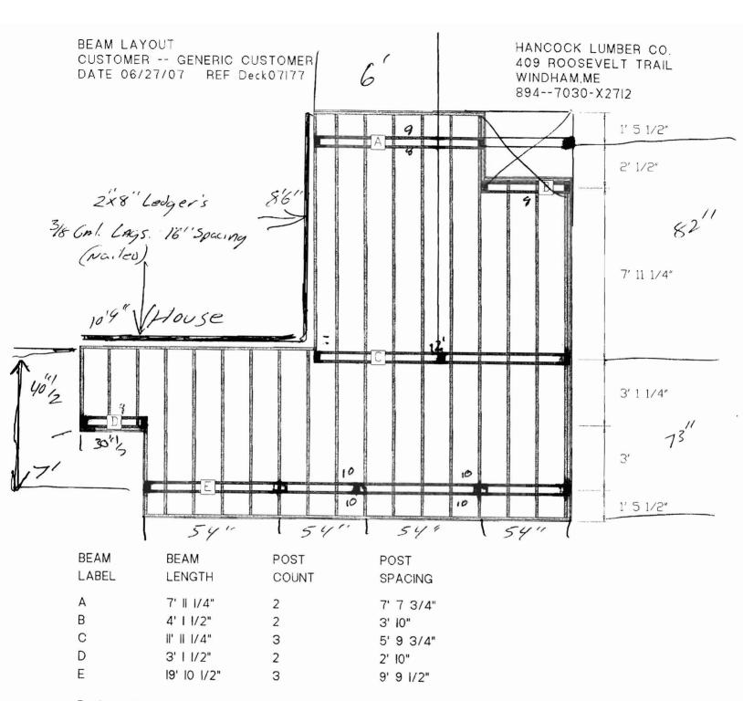
Post spacing is measured center-to-center.
