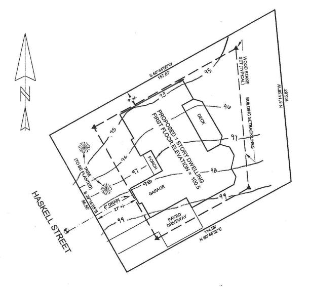
1.) THIS IS NOT A STANDARD BOUNDARY SURVEY. THIS PLAN IS COMPILED FROM SURVEY PLANS SUPPLIED BY ROBERT P. BURKEHARDT TO THIS SURVEYOR. THE WOOD STAKES SHOWN ON THIS PLAN WILL BE SET BY THIS SURVEYOR TO SHOW THE BUILDING SETBACK LINES.
