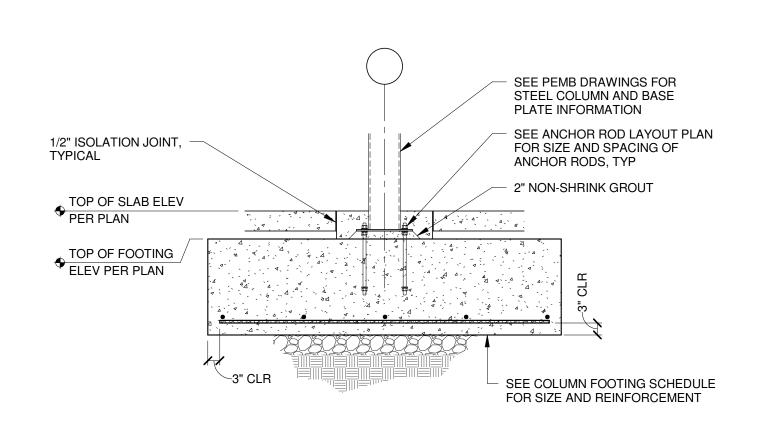
1. ANCHOR RODS SHALL BE SET AND HELD IN POSITION TEMPLATE WHICH IS LATERALLY STABLE AND WHICH PREVENTS ANCHOR RODS FROM BEING DISPLACED OUT-OF-PLUMB DURING CONCRETE PLACEMENT
