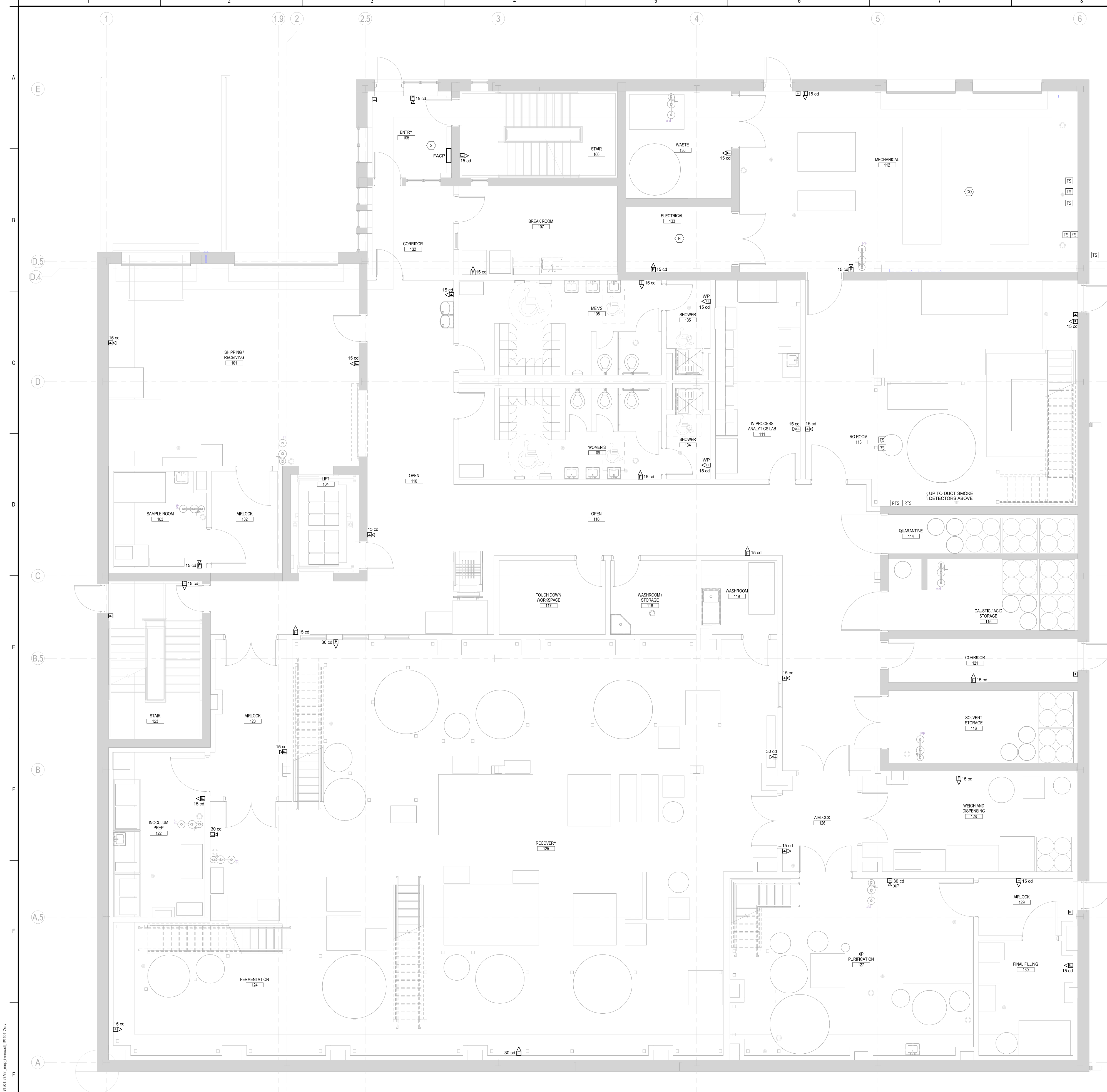
1 E-401-C FIRST FLOOR - FIRE ALARM PLAN 1/4" = 1'-0"
