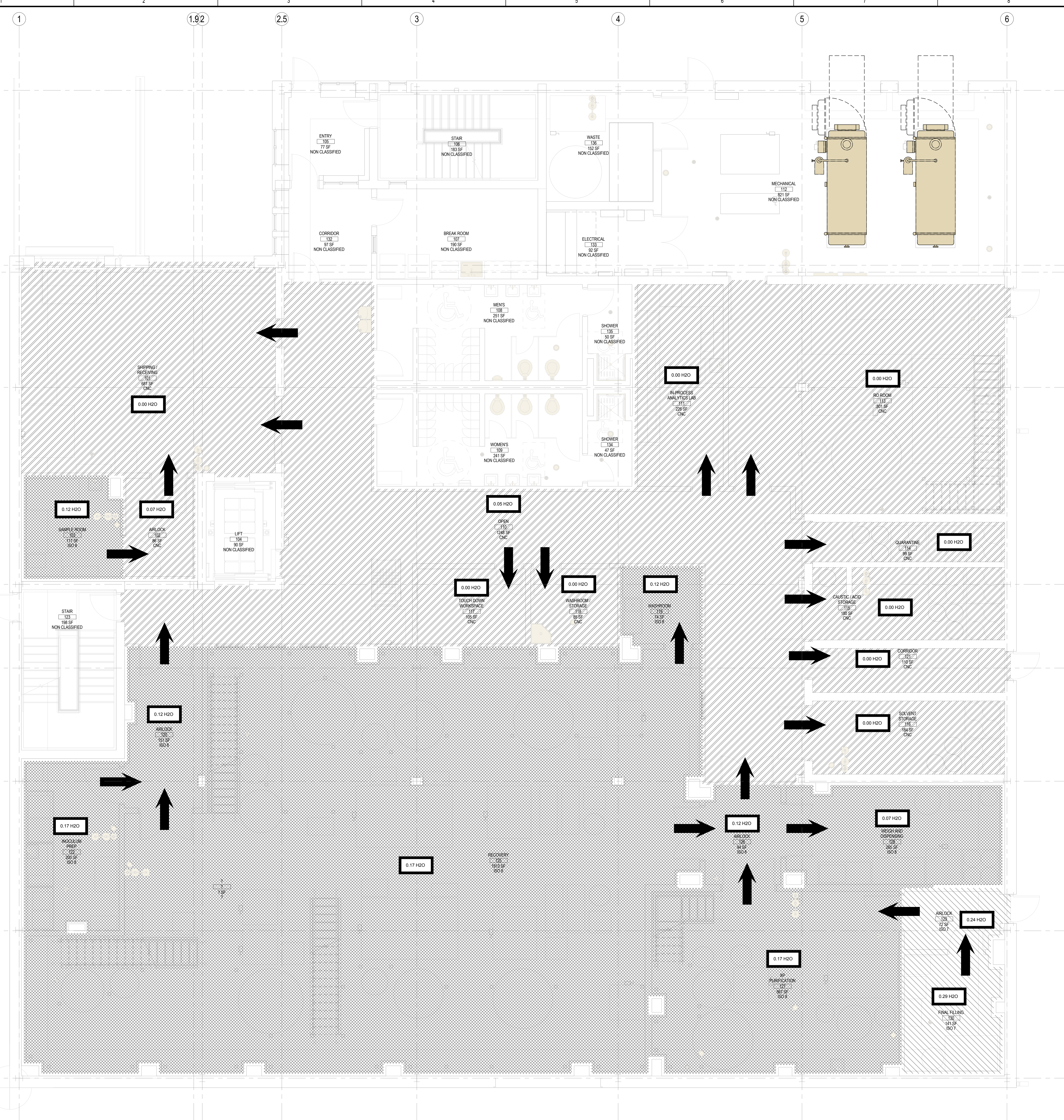
1 FIRST FLOOR - PRESSURIZATION CLASSIFICATION 1/4" = 1'-0"
