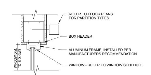
1 METAL STUD WALL WINDOW HEAD DETAIL
