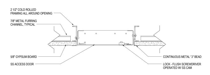
SUSPENDED GYP. CEILING ACCESS PANEL DETAIL
