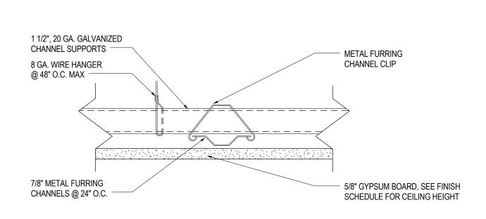
7 SUSPENDED GYPSUM BOARD CEILING DETAIL, TYPICAL
