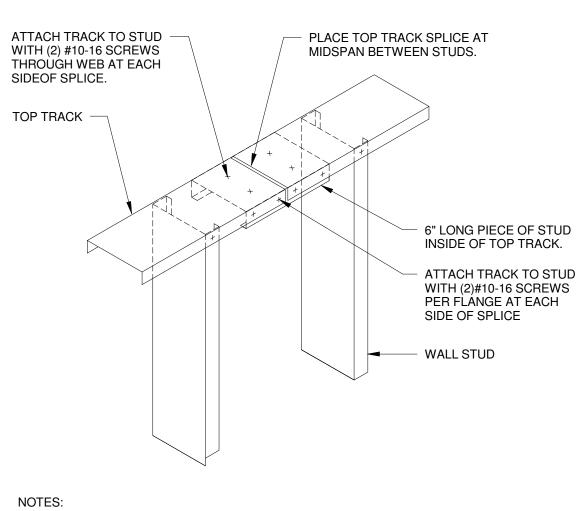
1. DO NOT SPLICE TRACKS (TOP OR BOTTOM) WITHIN 2'-0" OF THE X-BRACE
