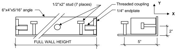
This insert is used on the vertical sides of the endwalls. The 4" leg forms the outside edge of the endwalls, and the 6" leg is abutted to the side walls and is used for the welded connection to the side wall, the roof, and the floor.
