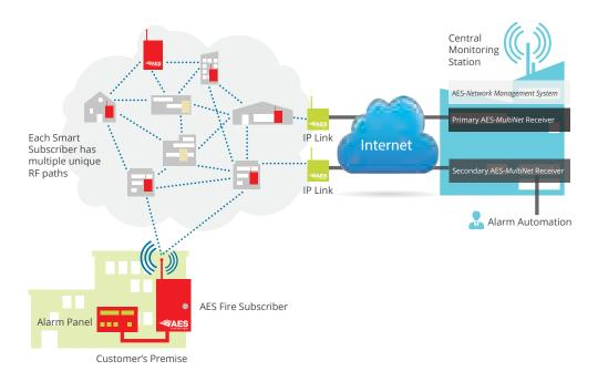
Each Smart Subscriber acts as transmitter, receiver, and repeater creating a smart long-range radio network with multiple pathways and multiple redundancies. The AES-*IntelliNet* network is self-forming, self-healing, highly scalable and assures that signals follow the shortest path available as the network expands.
