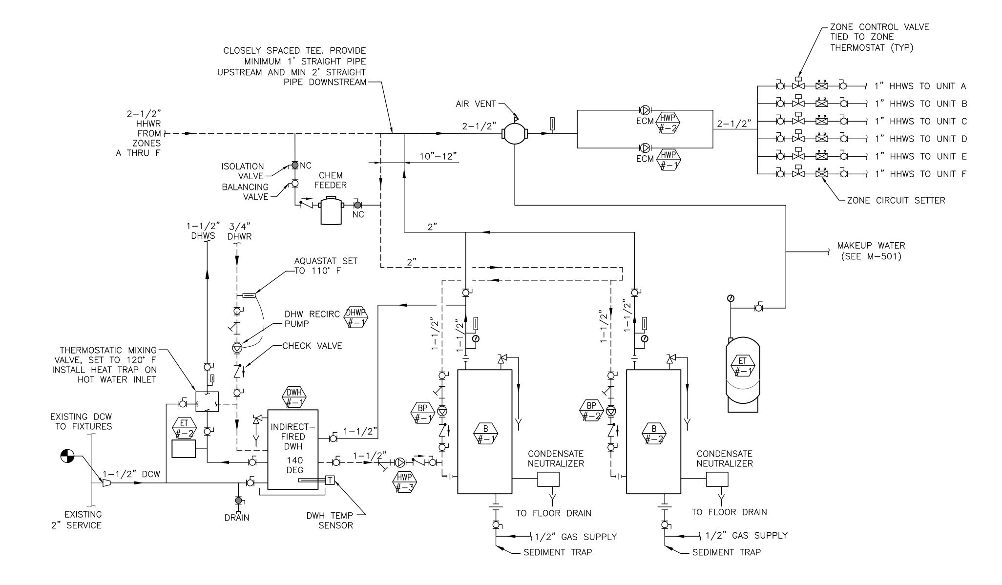
HEATING & DOMESTIC HOT WATER SCHEMATIC SCALE: NTS
