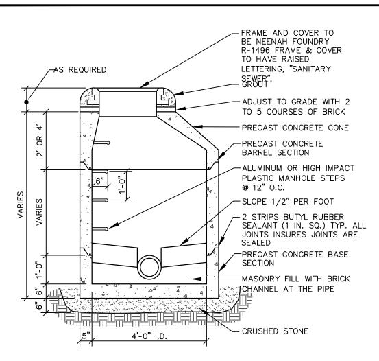
NOTE: PIPE CONNECTIONS SHALL BE WATERTIGHT FLEXIBLE BOOT CONNECTORS PROVIDES LEAKPROOF CONNECTION
